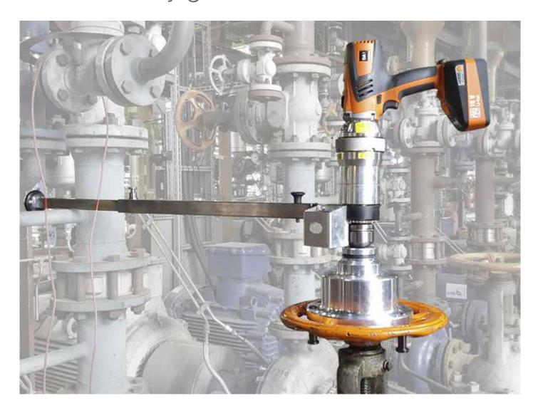
The Plarad DA1-05 S battery gate valve wrench is used for opening and closing of any valves as butterfly valves, ball valves or gate valves. The Plarad DA1-05 S can be optimised for specific applications by adapting additional accessories.
